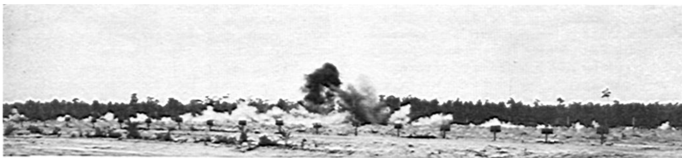
.05 second delay fuze; height of burst: 8 feet
