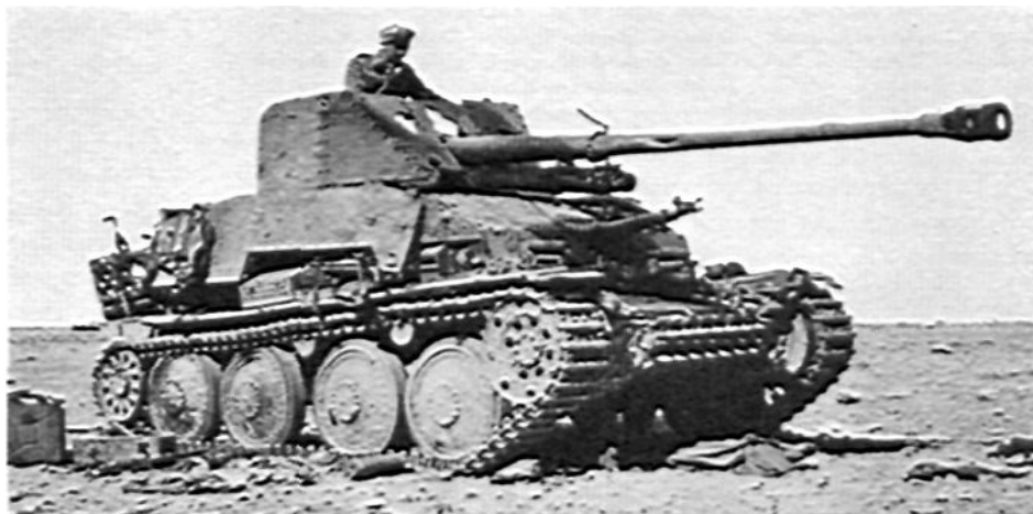
The Germans have mounted Russian 76.2-mm. AT guns on Czech T.N.H.P. light (10-ton) tanks, for use in Africa.
