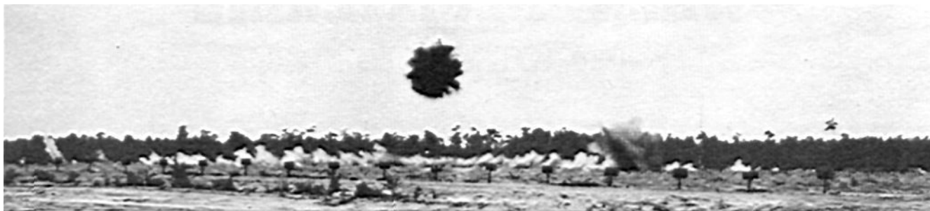
.15 second delay fuze; height of burst: 24 feet
